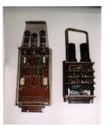
The new (l) – constructed by me - and the old, originally (r) logic units of the M-3 computer:
