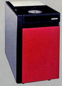
DM-312 Single Density Drive. The Ampex DM-312 is a single density 29 megabyte drive which is functionally equivalent to IBM drives using 2316 or equivalent disk packs. It includes a front panel select plug to change the unit number dynamically by interchanging plugs. The format is 200 cylinders with four alternates.
