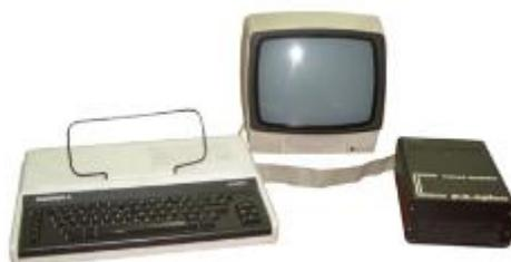
**Figure 1.** Elwro 800 Junior: microcomputer, screen, tape recorder
